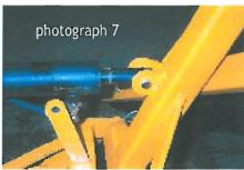
the pins out of the transport brackets, photograph 6, and replace them through the rams with the clips and pins, photograph 7.
