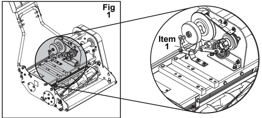
Under tensioning this belt will lead to slip and cause rapid wear. Over tension will put excessive strain on the belt and bearings.
